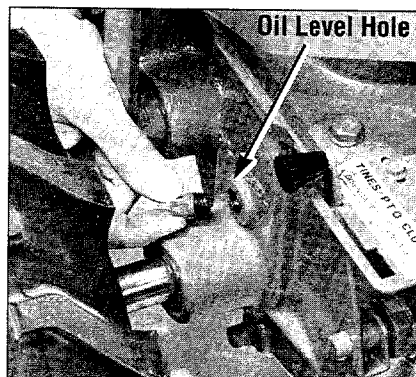
Photo 2-16: Gear oil should seep out from oil level check hole in power unit transmission.
